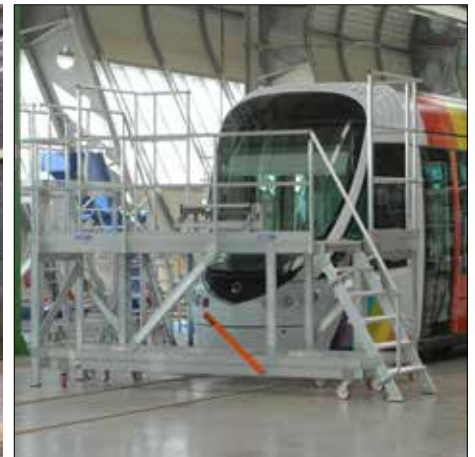
Work Platform Surround for Rail/Passenger Vehicles
