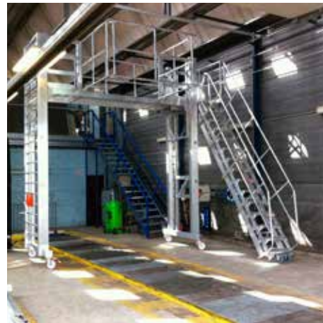
Overhead Gantry & Inspection Platform for Large Vehicles
