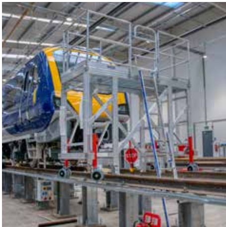
Railway Windscreen Access Platform
