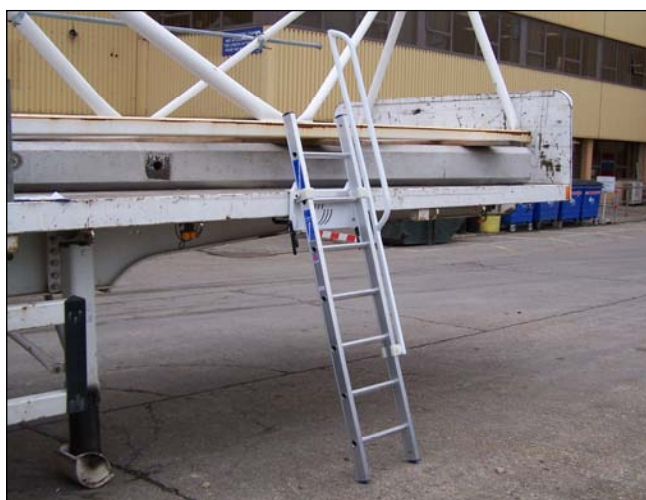
Figure 1 Ladder in use on flat-bed trailer
