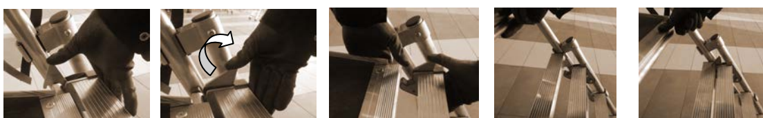
Unlock the hook with your right hand. Take hold of the platform with your left hand and raise so that the hook is lowered below the bottom step.
