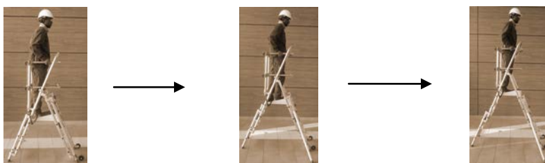
The stabilizer is put in place by unlocking the cam. It is in place once it makes contact with the floor. The cam must then be locked in position before the unit can be used.
