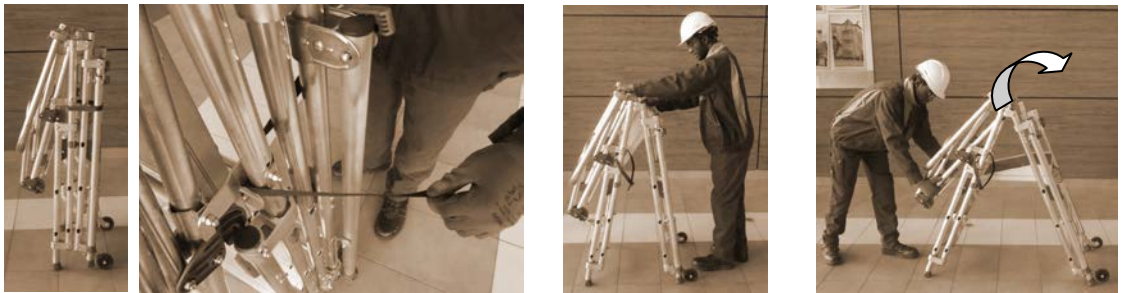
Undo the velcro fastener and unfold the platform by lowering it
