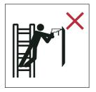
Avoid work that imposes a sideways load on ladders, such as side-on drilling through solid materials.
