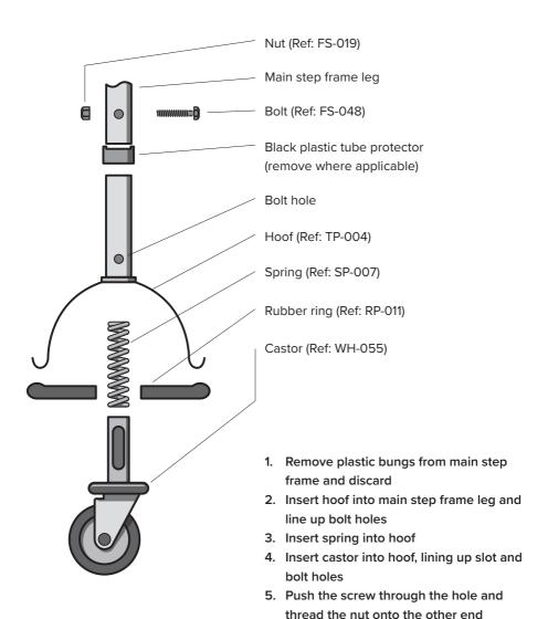
6. Tighten using a slotted screw driver
