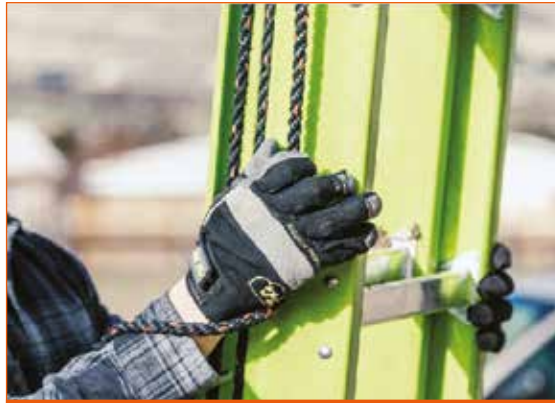
Side mounted, heavy-duty rope operated ladder reduces effort needed by 45%
