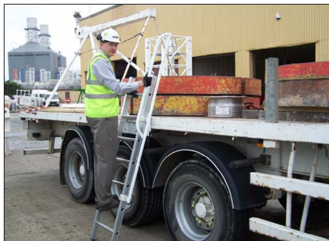
Figure 3 Access system in use
